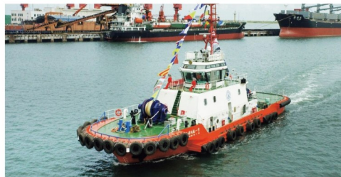
“云港电拖一号”4000HP纯电动拖轮
